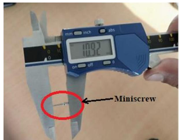
Fig 2. Measurement on Digital Caliper
