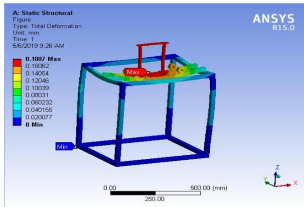
Figure 3: Total deformation in frame
