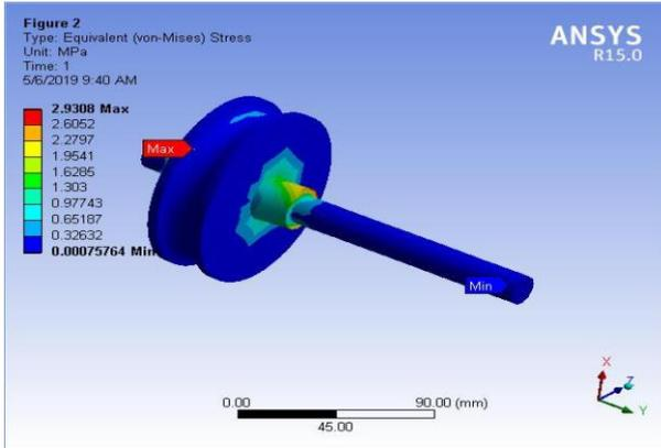
Figure 4: Equivalent stresses acting in rollers
