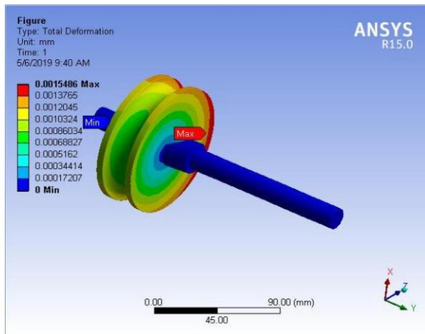
Figure 5: Total Deformation in rollers
