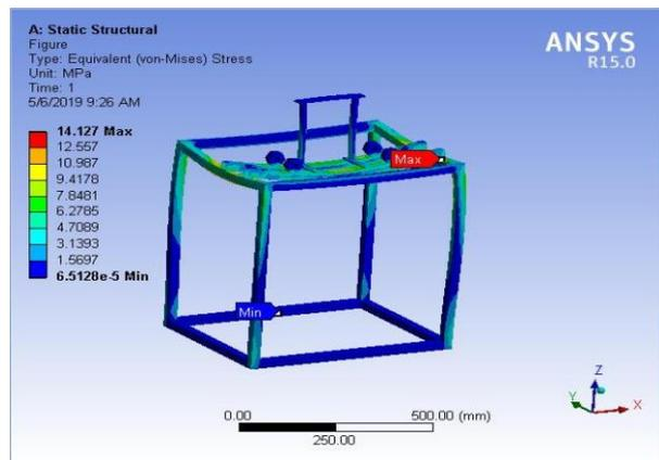
Figure 2: Equivalent stresses acting on frame
