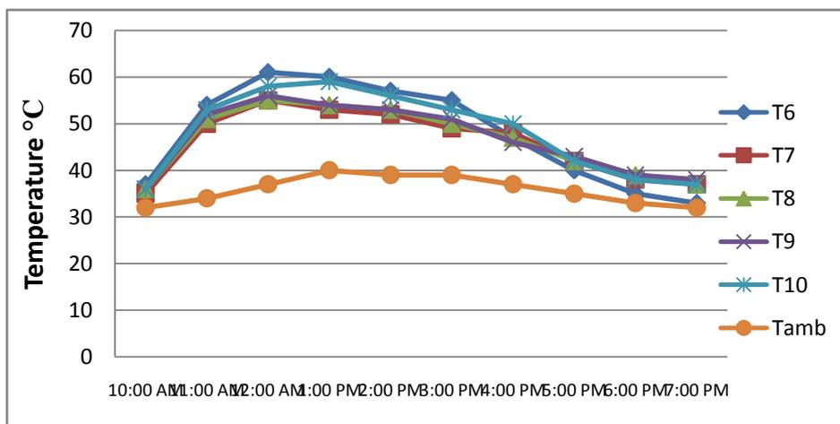
Fig 5: Variation of cabinet temperatures and ambient temperature vs. time for day 1
