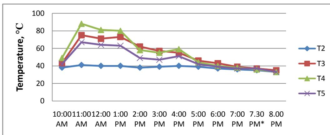
Fig 9: Variation of collector temperatures and gravel stones vs. time for day 1
