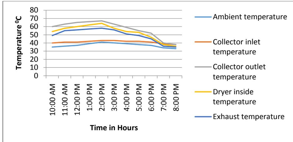
Fig. 3: Variation of temperature at various locations during Test -2 of day-1
