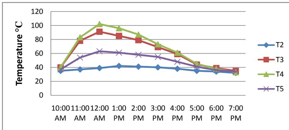
Fig 4: Variation of collector temperatures and gravel stones vs. time for day 1
