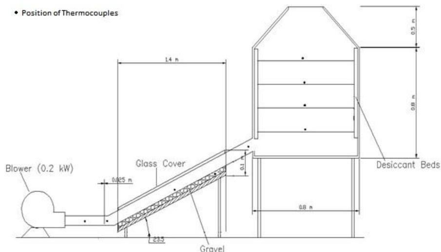
Fig 1: Schematic diagram of the experimental setup
