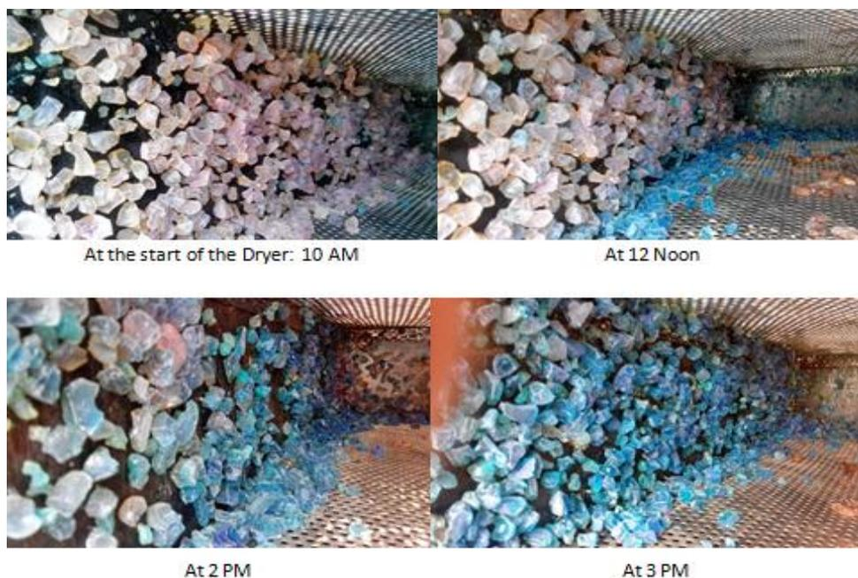
Fig 11: Desiccant beds adsorption and regeneration
