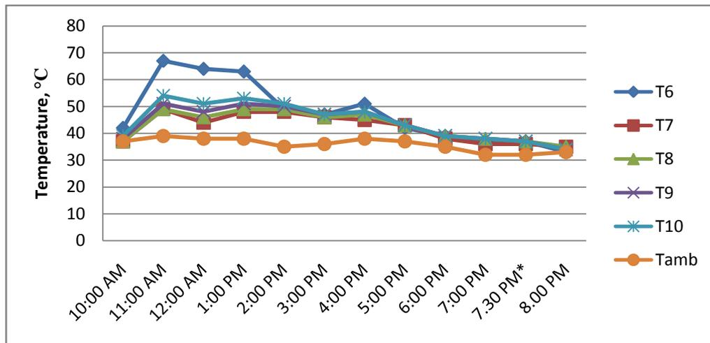
Fig 10: Variation of cabinet temperatures and ambient temperature vs. time for day 1
