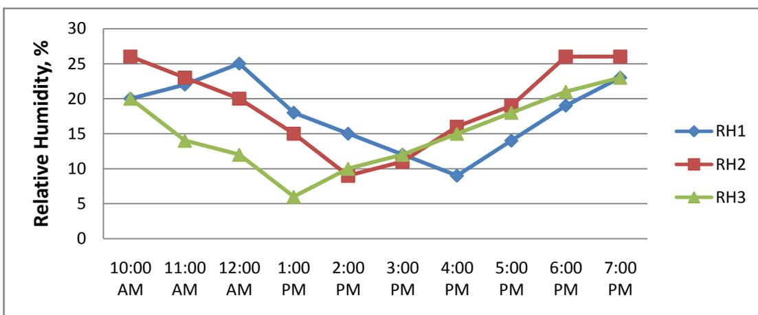
Fig 14: Variation of dryer relative humidity for 3 days
