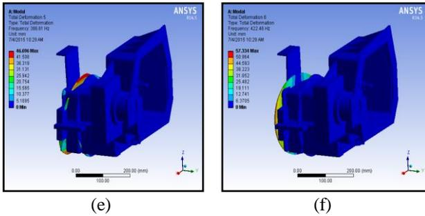
Figure 6. Different mode shapes at different 6 natural frequencies after structural modification
