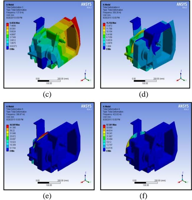
Figure 5. Different modes of vibration at first 6 natural frequencies
