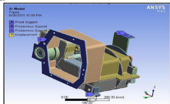
Figure 2. Meshed Geometry of Gearbox
