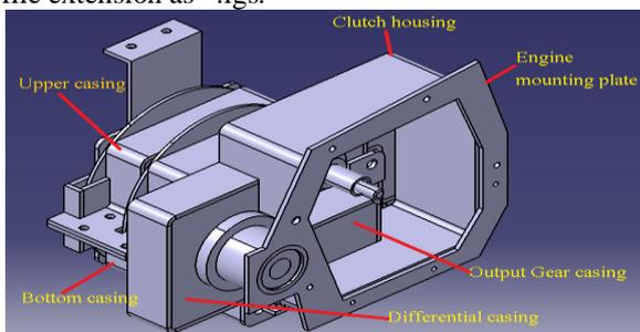
Figure 1. Geometry of Gearbox Casing
