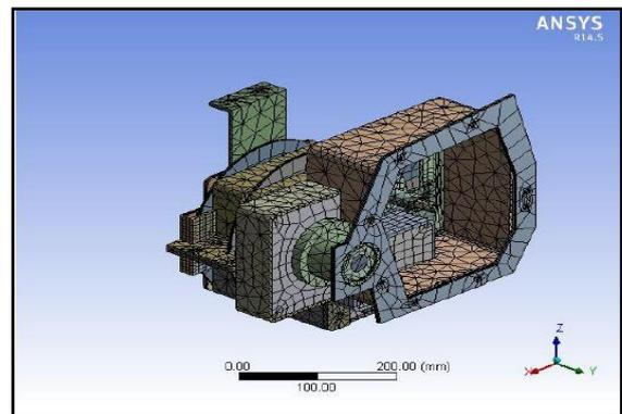
Figure 2. Meshed Geometry of Gearbox
