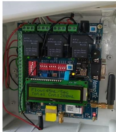
Fig 5: Water Supply Counting Display
