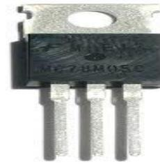
Fig.4 : 7805 voltage regulator IC
