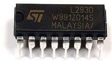
Fig.7: L293D Relay/Motor
