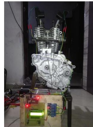
Fig9: Solenoidal Valve Actuation System for Four Stroke IC Engine
